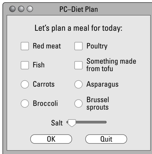
Figure 5-1: Creating a Visual Basic or REALbasic program involves placing controls on a window.
